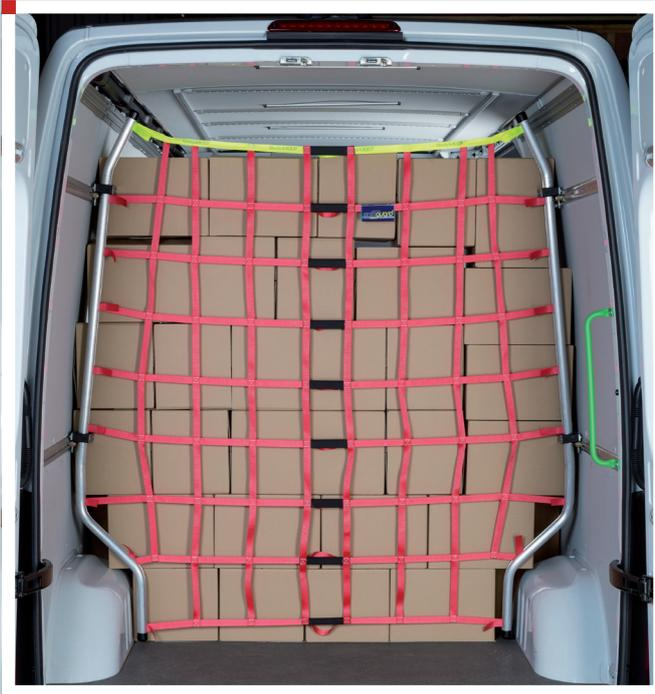
The innovative QuickKEP safeguard load securing net was designed for **fast** and **safe handling**.
